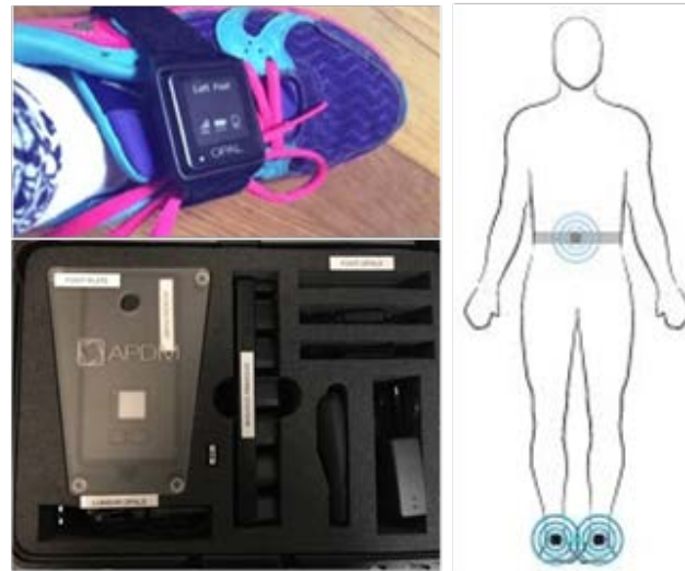
OPAL sensor, kit and placement for testing gait and balance
